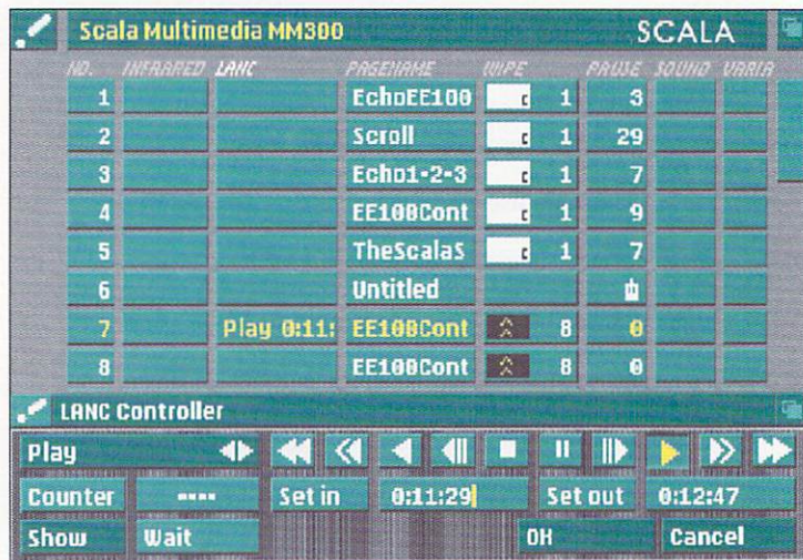
When you edit with Scala Echo, you use the Scala MM300 interface. At bottom, Echo's LANC control panel sports VCR-like buttons that control the source VCR.
